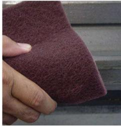
Surface finishing hand pads are made of a non-woven nylon web impregnated with abrasive grain and resin bond.
